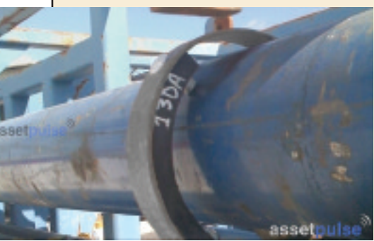
Close up of the bracket that connects the RFID tag to the pipe, and, above, a demonstration of how robust the attachment is.
